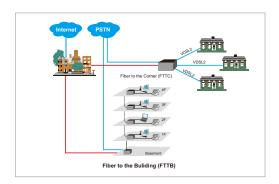
The VDSL2 technology is also deployed at the last mile of internet access. The ISP uses the fiber cable as backbone uplink to the basement of building (FTTB) or corner of streets (FTTC) and uses the existing 1 pair twisted cable of POTS system to carry voice and Ethernet data stream to users via VDSL2 signal.
